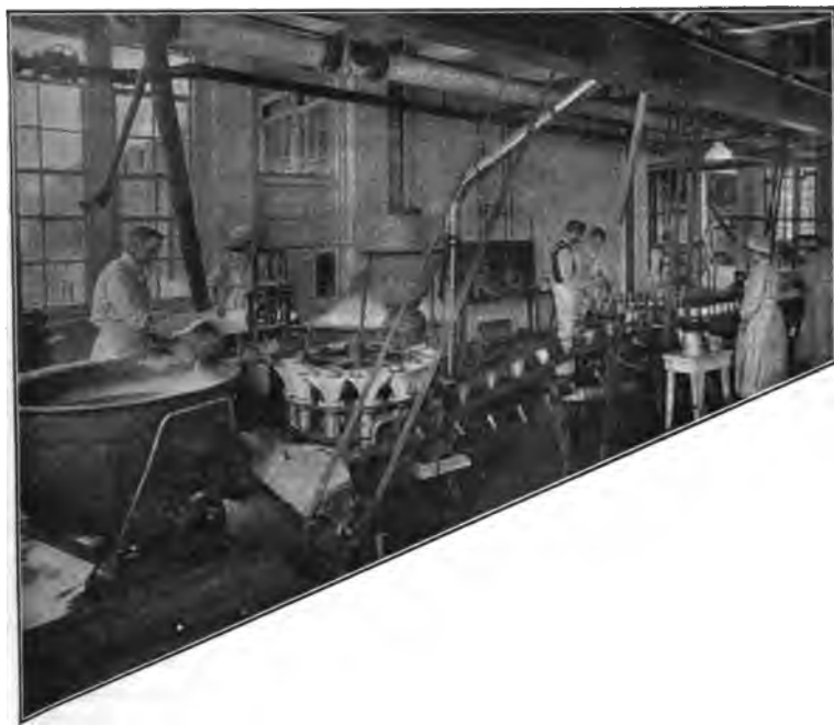
FIG. 66.—Cans of food filled by machinery and automatically carried past inspectors, finishers, and solderers who complete the closing of the cans. (Joseph Campbell Co., Camden, N. J.)
